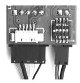
Small white connector on back of transmitter is for ImmersionRC Tiny Telemetry. See accessories.
